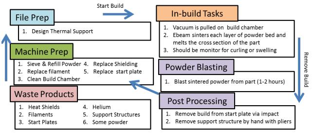
Figure 3: Process cycle for operating EBM system
