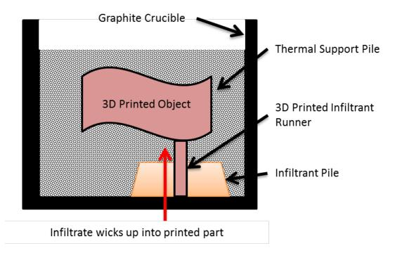
Figure 5: Setup configuration for the sintering and infiltration of I-3D printed green parts
