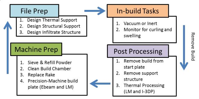
Figure 1: Basic metal powder bed AM process flow
