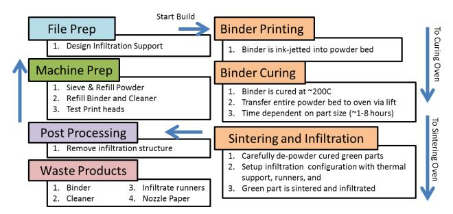
Figure 4: Process cycle for binder jetting
