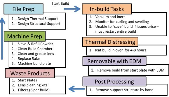
Figure 2: Process cycle for LM
