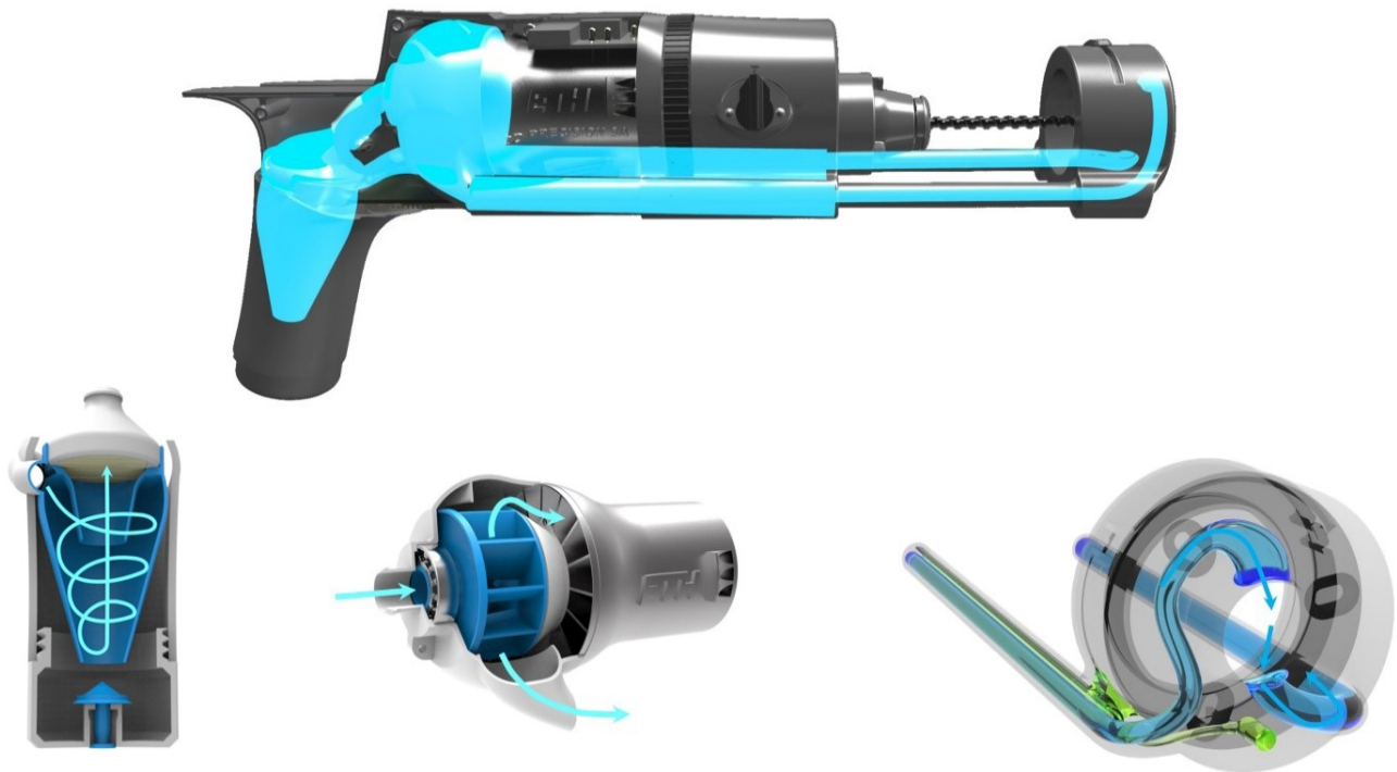
Figure 6: Overview of ventilation and dust extraction system (above), cyclonic separator (left), centrifugal fan with motor cooling (middle) and dust extraction base (right).
