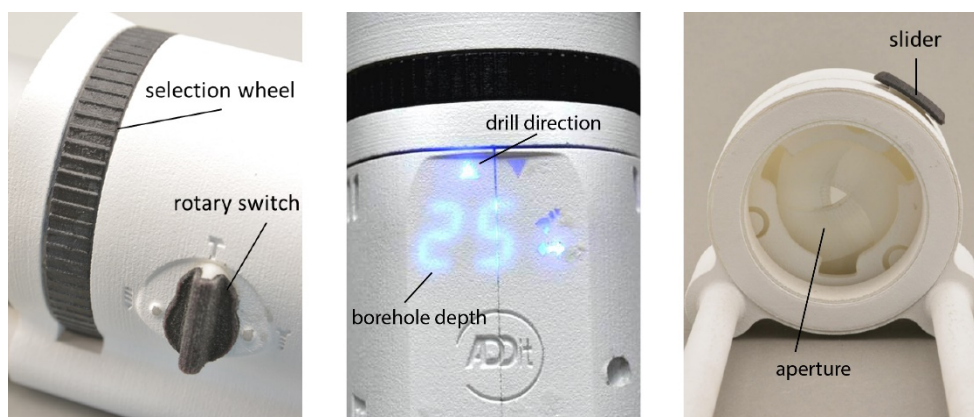
Figure 3: Selection wheel and rotary switch (left), display (middle), dust extraction base with aperture (right)
