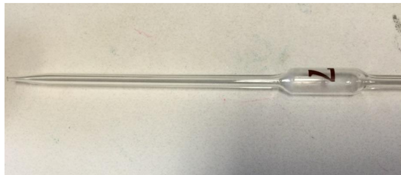
Figure. 5 Volumetric pipet used for measuring the surface tension of the binder
