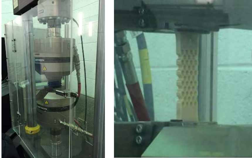
Figure 6. The INSTRON 8801 setup for compression testing (left) and tension testing (right)
