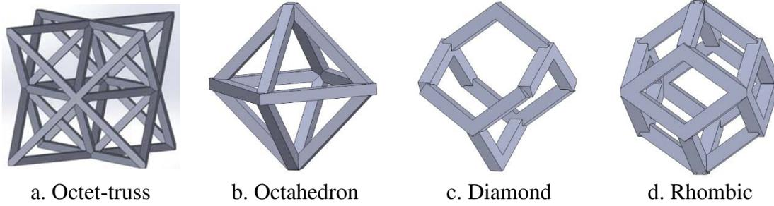
Fig.5 Several unit cell designs with cubic GBV
