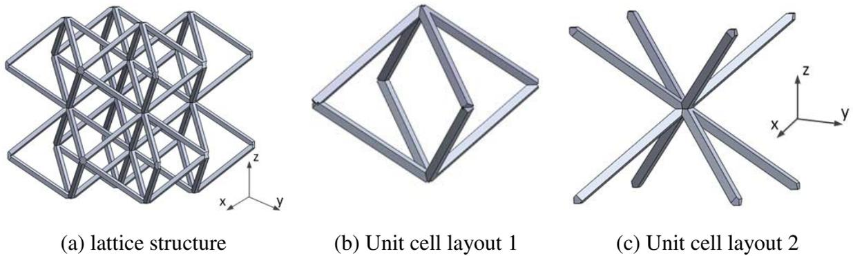
Fig.6 BCC lattice cellular structure [26]
