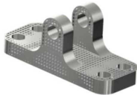
Figure 9: Load dependent optimization of lattice density [LC15]
