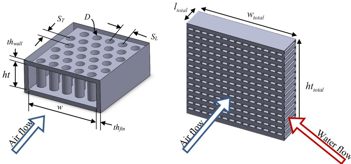
**Figure 1:** Geometric configuration. Left: air-side microstructure. Right: macrostructure.
