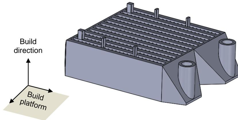
**Figure 2:** Representation of print orientation.
