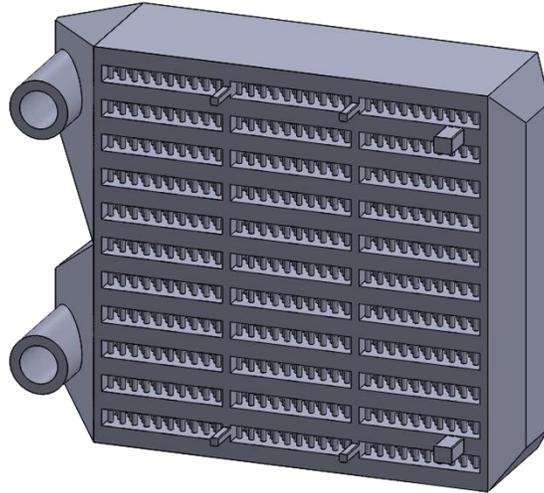
**Figure 5:** Prototype heat exchanger printed using material extrusion with ABS.
