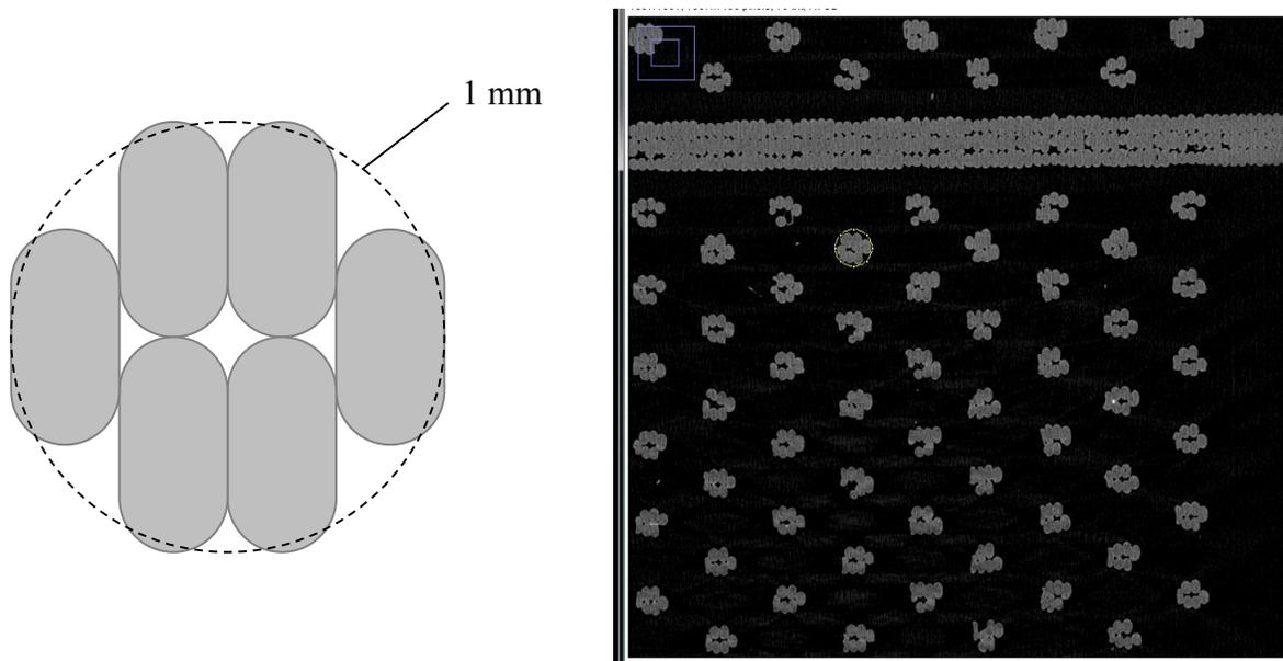
**Figure 4:** Cross-sectional view of pin fin array in CT scan.
