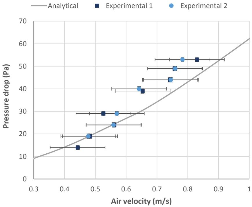
**Figure 7:** Experimental air-side pressure data.
