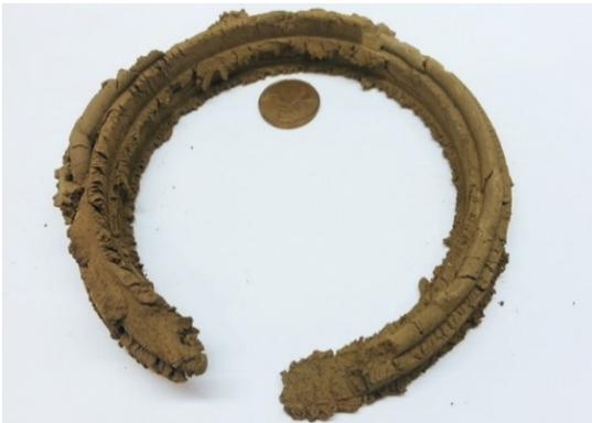
(a) Extruded sample with cracks on surface
