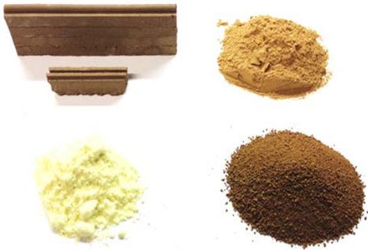
Figure 3 Martian regolith simulant sulfur concrete
