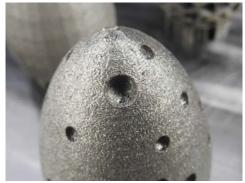
Figure 10: Example of an untreated surface illustrating a rough but glossy surface
