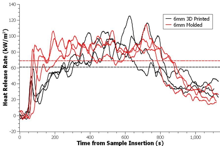
Figure 8: ASTM-E1354 cone calorimeter results for 6mm thick AM and molded ULTEM™ 9085 sheets at 40 kW/m<sup>2</sup> irradiance. Only the first 1150 s of data are shown. The mean average heat release rate for the first 1000 s is plotted as a dashed line, with the mean average heat release rate of the 3D printed and molded sheets being 61 kW/m<sup>2</sup> and 69 kW/m<sup>2</sup>, respectively.
