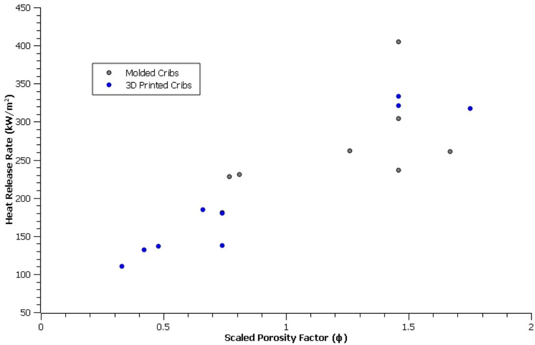
Figure 10: ABS crib pre-collapse heat release rate are graphed as a function of Block's porosity factor. The cribs were tested at  $40 \text{ kW/m}^2$  irradiance, and both molded and AM produced materials are included in the graph.
