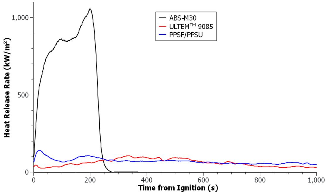
Figure 5: ASTM-E1354 cone calorimeter results for three additively manufactured polymer sheets. Testing was done at 40 kW/m<sup>2</sup> irradiance. Flaming for PPSF and ULTEM™ samples did not cease until 1700 s, but steadily decreased during that portion.
