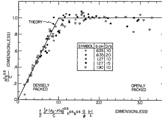
Figure 2: Block's experimental burning rate data scaled by porosity factor[17]
