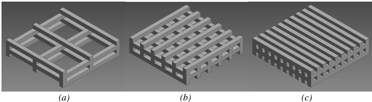
Figure 11: Cribs used in porosity study, using ABS material; (a) Porosity factor  $\phi = 1.46$ , (b)  $\phi = 0.81$ , (c)  $\phi = 0.33$
