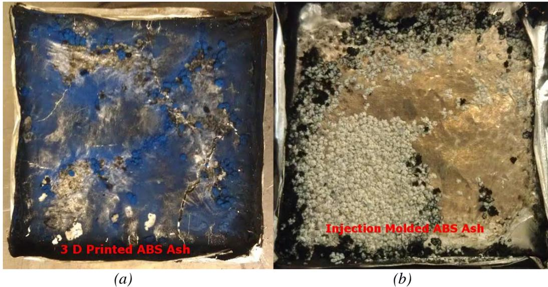
Figure 7: ABS sheet combustion ash: (a) AM sheet ash, (b) Injection molded sheet ash.
