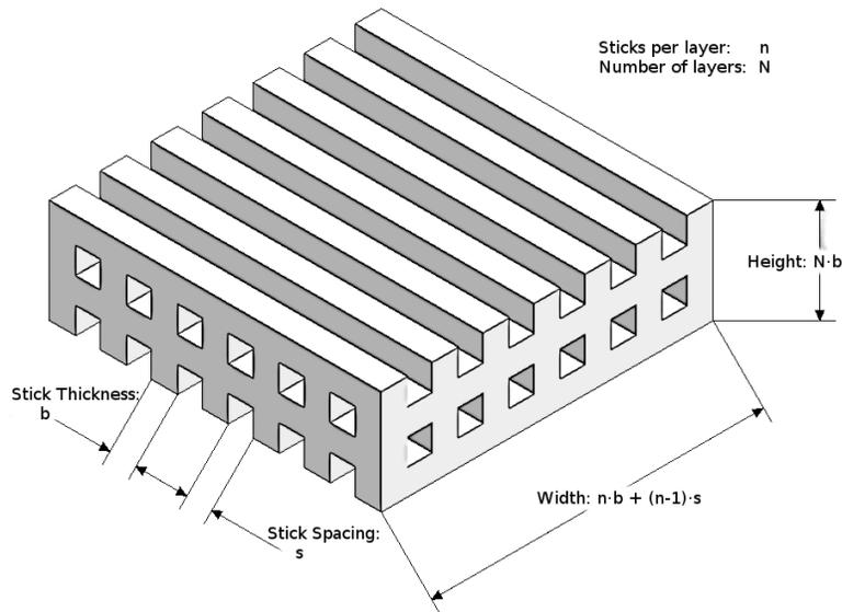
Figure 1: *Crib structure with parameters: square prism (or stick) member has thickness  $b$ , spacing  $s$  between sticks, number of sticks per layer is  $n$ , and number of layers  $N$  (the pictured example 4 layers with 7 sticks)*
