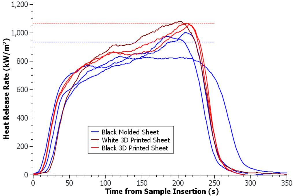
Figure 6: ASTM-E1354 cone calorimeter results for 6mm thick 3D printed and molded ABS sheets at 40 kW/m<sup>2</sup> irradiance. The mean peak heat release rate for the 3D printed and molded sheets are represented as the dashed lines in the figure. The average for the 3D printed and molded sheets are 1067 kW/m<sup>2</sup> and 933 kW/m<sup>2</sup>, respectively
