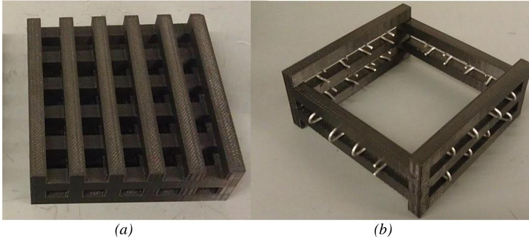
Figure 4: Additively manufactured ABS cribs. (a) The specimen is four layers and six prisms per layer, and the stick thickness is 8 mm. The porosity factor was calculated to be 0.74. (b) The specimen is five layers and two prisms per layer, supported by galvanized steel wire. The stick thickness is 6 mm. The porosity factor was calculated to be 1.75.
