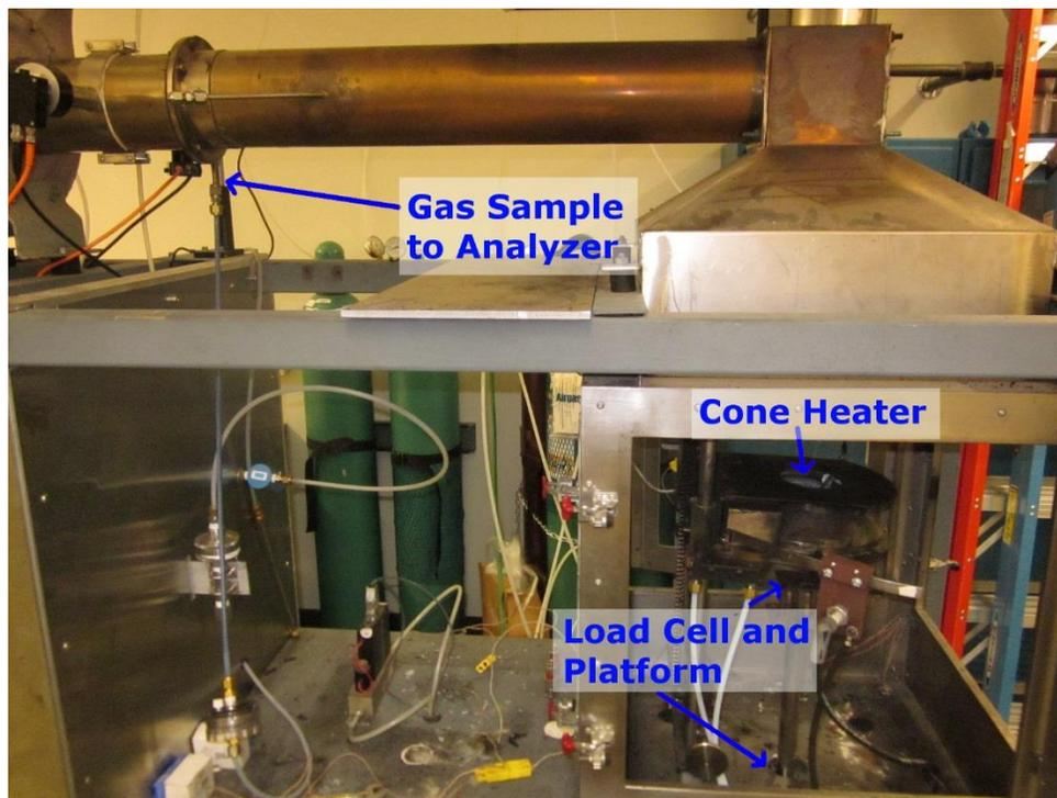
Figure 3: This photo shows the cone calorimeter used in the ExtReMe Lab at Virginia Tech. The major components are identified in the photo. Crib samples are placed on the sample holder under the cone heater for testing. Tests are performed to ASTM E1354.
