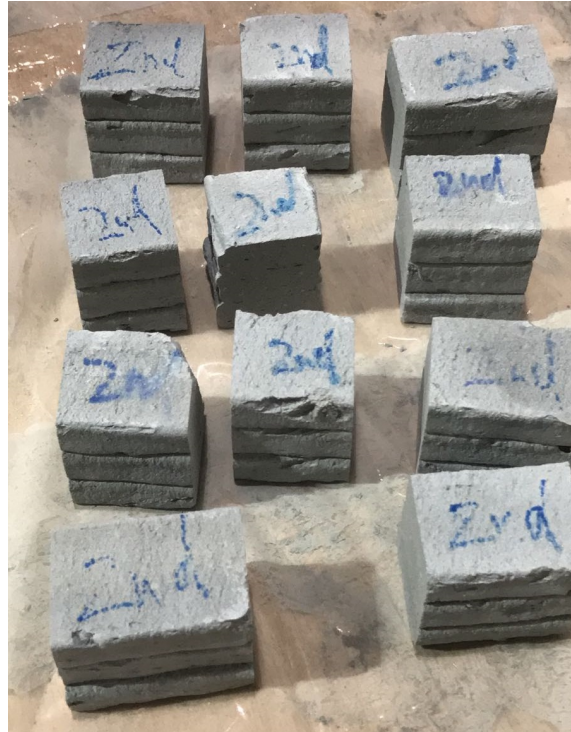
Figure 4: The cut pieces of sample printed by the second generation nozzle.
