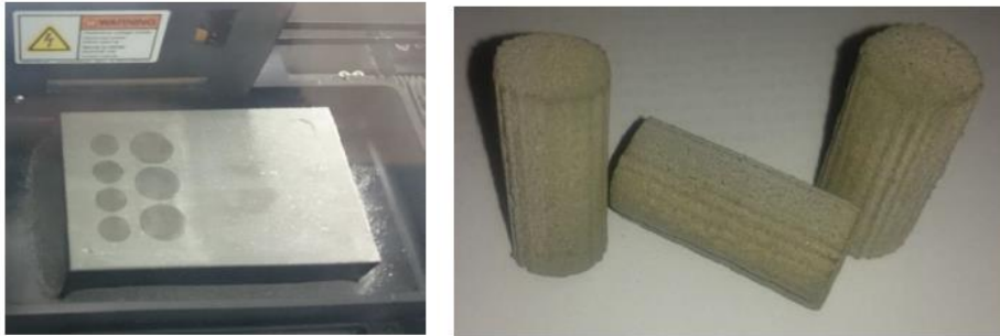
Fig. 4: Samples while being printed and after the sintering and after machining
