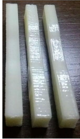
Figure 7 – Polishing effect as a function of number of repetition cycles
