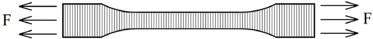
Figure 2. Layers result of printing in Z direction
