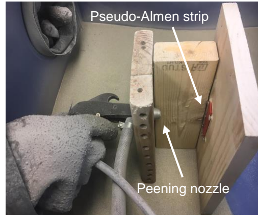
Fig. 9 Shot peening fixture.
