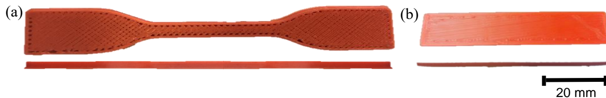
Fig. 4 Sample geometry: (a) ASTM 638D Type IV and (b) pseudo-Almen strips.
