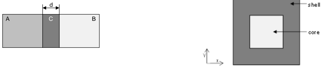
Figure 4: Left: Representation of overlap C between two different materials A and B; Right: Representation of building order in case of 3D Multi-material parts
