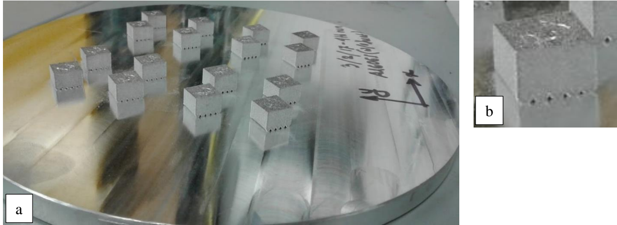
Fig. 4 LM-fabricated AA6061 cube parts (10 mm on each side) attached to the build plate (a). A closer view of one of the specimens is offered in (b).
