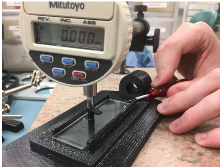
Figure 19 - Experimental setup to observe the elevation change of the slide as it travels horizontally
