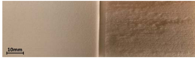
Fig. 1. SLS vertical wall surface finish. Side by side samples: standard finish (left) and orange peel (right).
