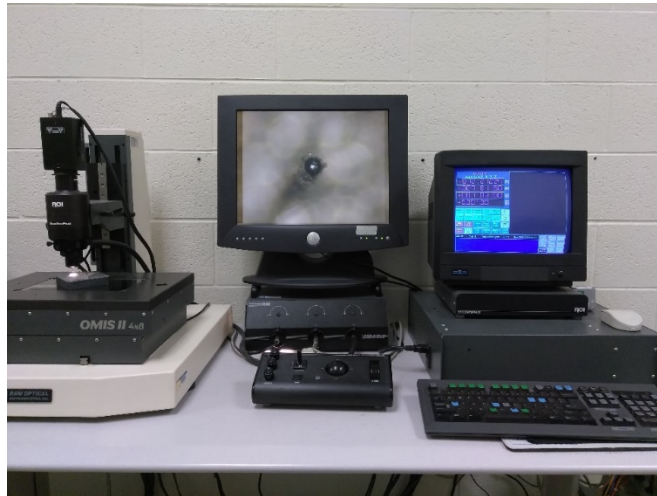
Figure 6. OMIS II optical measurement system inspecting fine feature.
