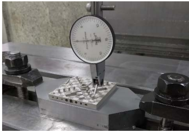
Figure 7. Dial indicator measuring pin height.
