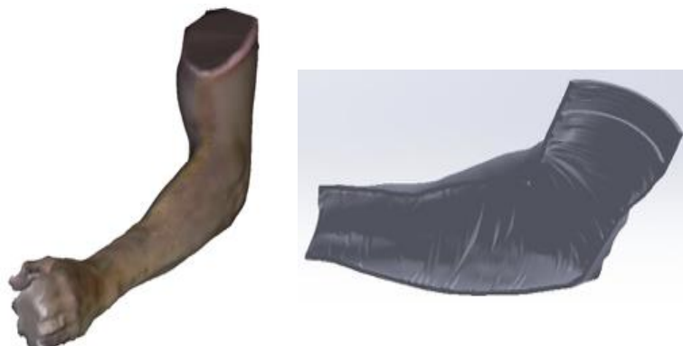
Figure 2. Raw scan from 3D Sense Scanner (left) and cross-sectional rendering of shelled, mirrored arm (right)
