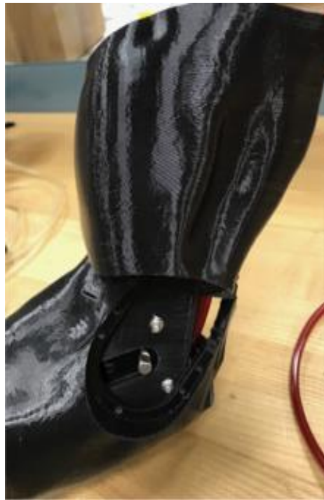
Figure 11. Model with interior mounting boss attachment removed to show actuator placement
