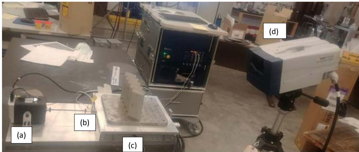
Fig. 10: LDV test setup. (a) Electrodynamic shaker; (b) Impedance transducer; (c) Air bearing platform; (d) Scanning LDV.
