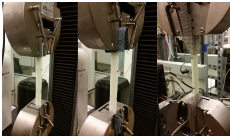
Figure 6: Specimen protection through tabbing. From left to right: No tabbing, emery cloth and wire mesh.
