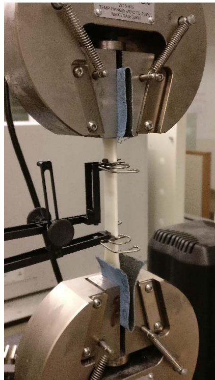
Figure 7: Test setup with 100 grit emery cloth protection and extensometer.
