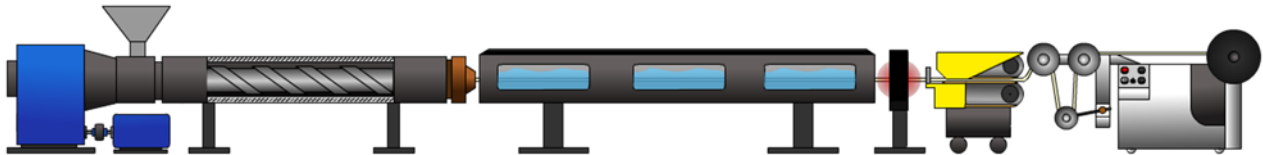
Figure 3: Extrusion setup schematic. From left to right: Extruder, Vacuum-assisted water bath, laser micrometer, puller, and filament winder.
