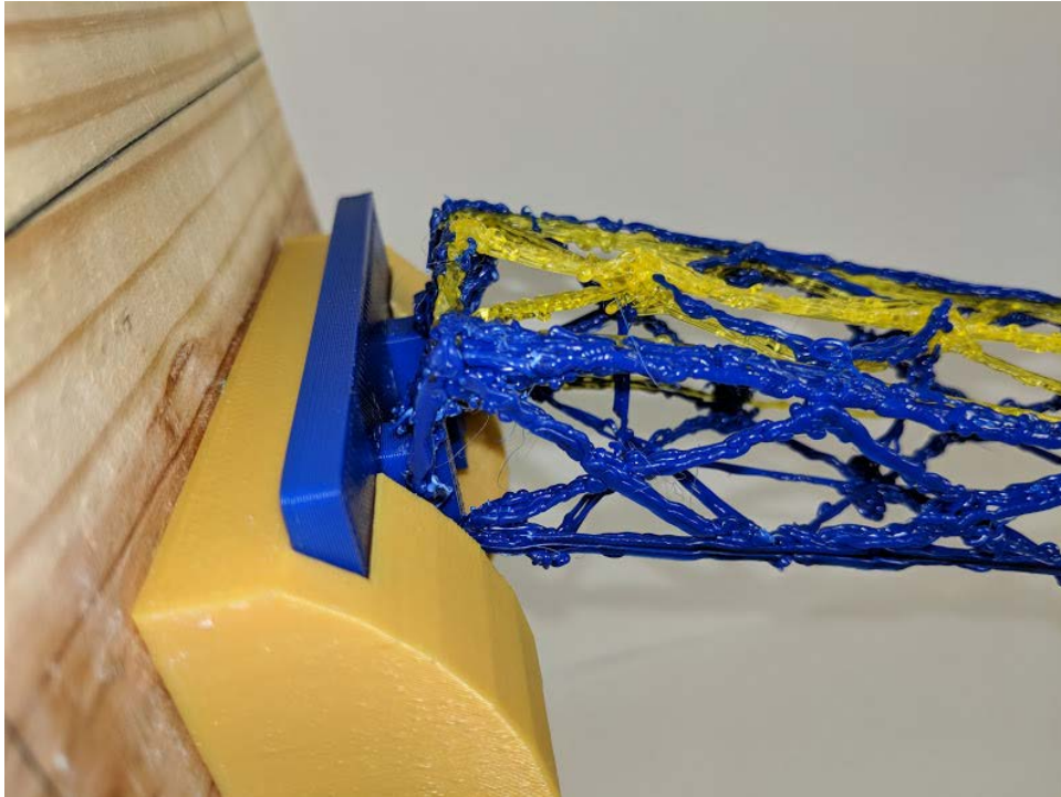
Figure 14 Wing-box with poor fused material at the attachment
