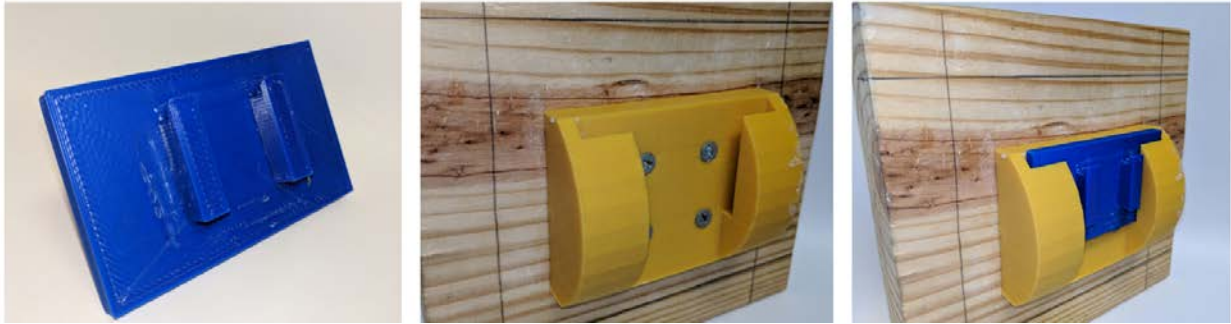
Figure 6 Attachment, base, and assembly for the wing-box testing
