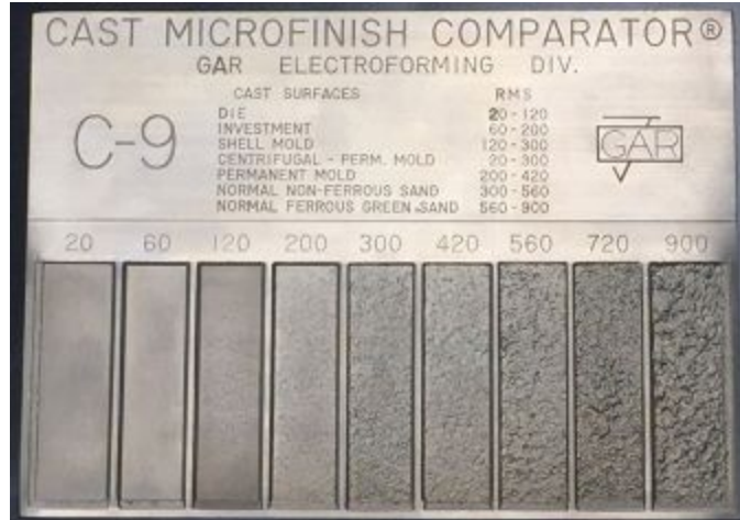
Figure 8: A cast microfinish comparator plate used to evaluate surface finish of the flat bar
