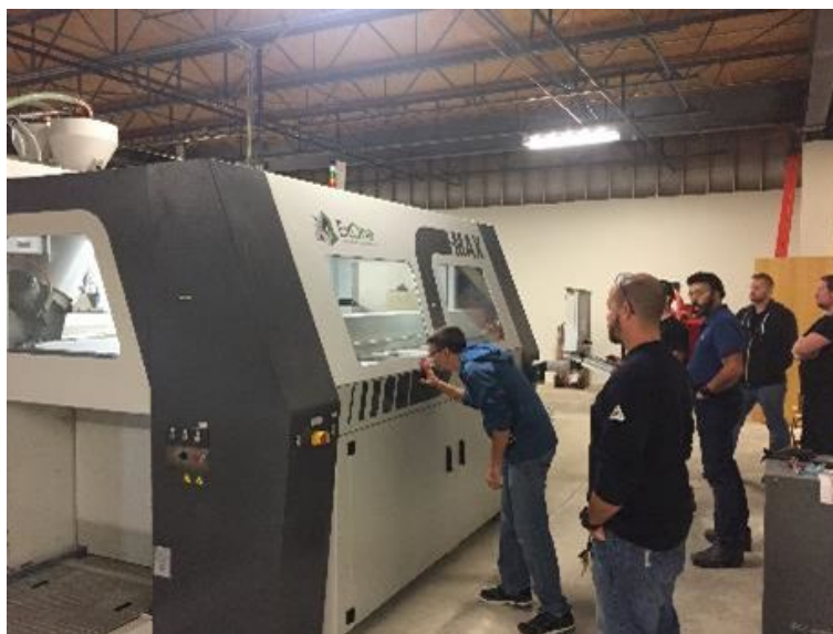
Figure 7: YSU's ExOne S-Max 3D sand printer
