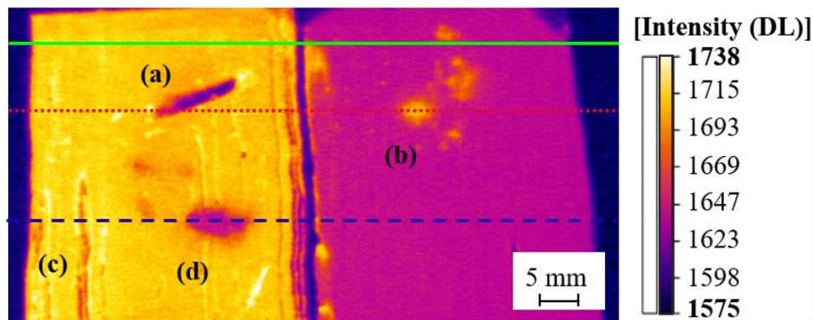
Figure 4: Result of multi-material powder layer monitoring. 1.2709 is applied on the left side and CuCr1Zr on the right. Section of the thermogram of a sample taken with following parameters: 640x512 pixel, 100 Hz frame rate, 0.0003 s integration time. The image represents the radiation 0.09 s after the excitation. (a) defect, (b) 1.2709 on CuCr1Zr, (c) groove and (d) CuCr1Zr on 1.2709. The colored lines in the image represent the positions of the line image analysis, shown later in Figure 5.
