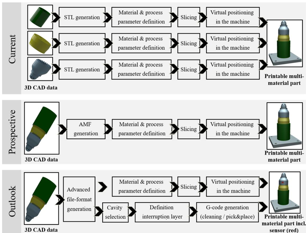
Figure 3: Data flowcharts for the production of mechatronic multi-material parts: current, prospective and outlook.
