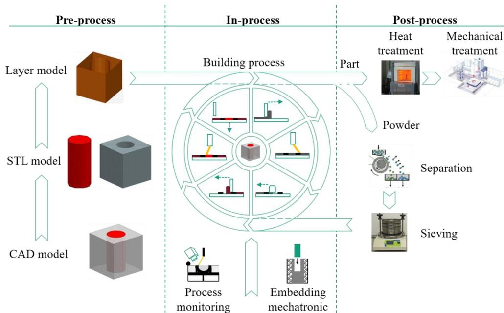
Figure 1: Process chain for (mechatronic) multi-material parts produced using LPBF
