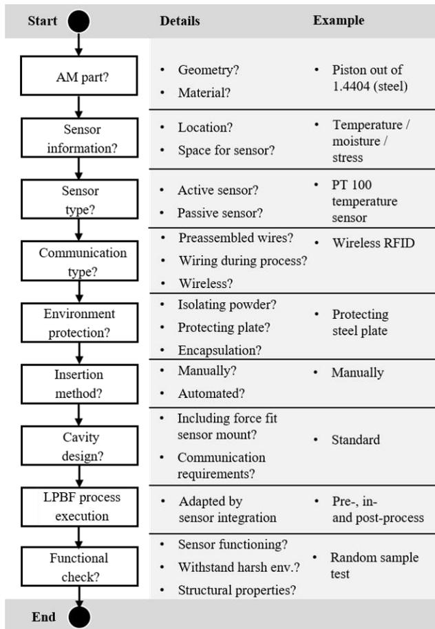
Figure 6: Procedure model for the integration of mechatronics into LPBF parts, using the example of sensor components
