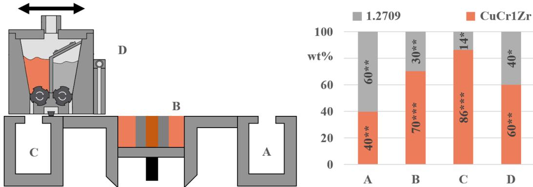
Figure 8: Schematic representation of the multi-material LPBF process chamber (left) and quantified results of the mixing ratio analysis of different positions within the process chamber (right). \*: 10 %  $\geq CV > 5\%$ ; \*\*: 5 %  $\geq CV > 1\%$ ; \*\*\*: 1 %  $\geq CV$ . The built part consists out of 50 wt% 1.2709 and 50 wt% CuCrZr.
