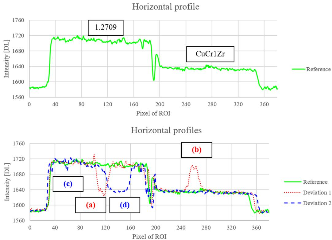
Figure 5: Intensity responses of thermographic pictures. The different graphs are linked to the linear image analysis positions shown in Figure 4. Upper diagram: Different intensity replies of CuCr1Zr and 1.2709. Lower diagram: Effects on the intensity reply caused by defects: (a) defect, (b) 1.2709 on CuCr1Zr, (c) groove and (d) CuCr1Zr on 1.2709.
