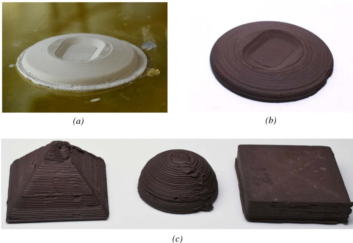
*Figure 5 – a: Green state Ø40mm conformal geometry having undergone post process machining operation. b: Conformal geometry post-thermal processing with a measured diameter of Ø33.2mm. c: a sintered pyramid, hollow hemisphere and tile that have been fabricated using the hybrid approach but have not been post processed using machining.*
