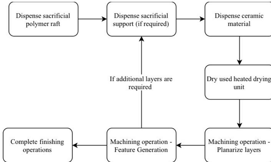
Figure 3 - Process flow demonstrating the production of a green state ceramic component
