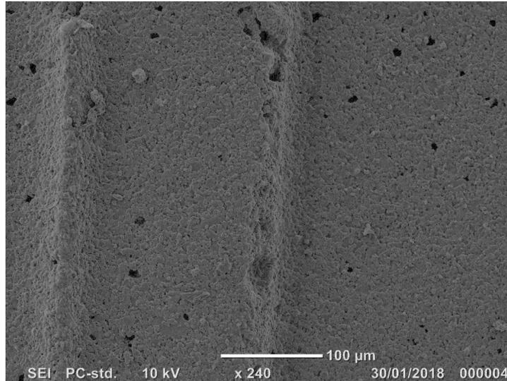
Figure 7 – SEM image of the interlayer region on a sintered part
