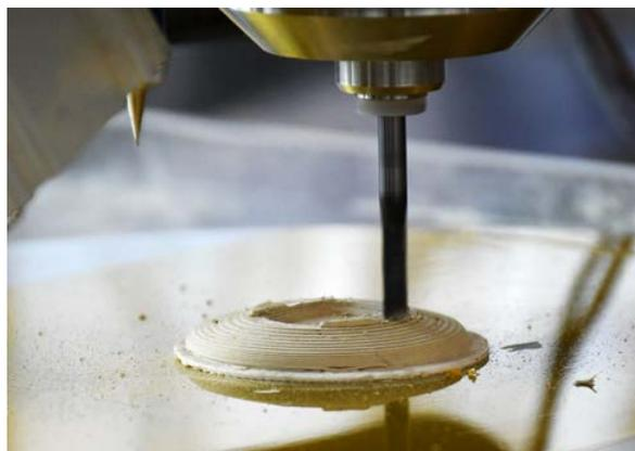
Figure 4 - Interlayer machining of a conformal geometry using a  $\text{\O}4\text{mm}$  CVD diamond end mill
