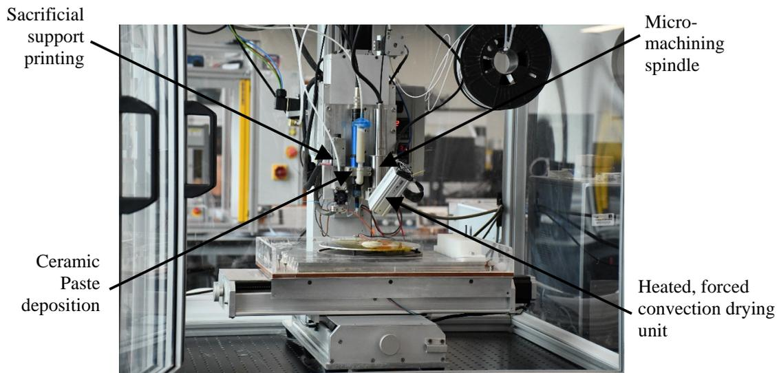
Figure 1 – Bespoke, digitally-driven manufacturing platform using a hybrid manufacturing approach
