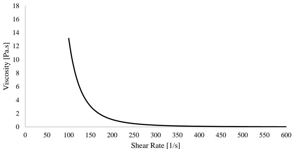
Figure 2 – Graph showing the results of the rheological tests on the paste
