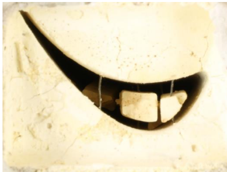
Figure 4. Mold after burnout showing a cracked core.
