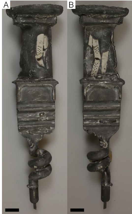
Figure 5. Optical photographs of an A356 turbine blade showing dislodged cores. Both scale bars are 1 cm.
