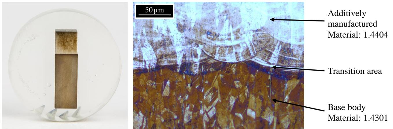
Figure 3: Micrograph of hybrid sample; macroscopic (left) and microscopic (right)
