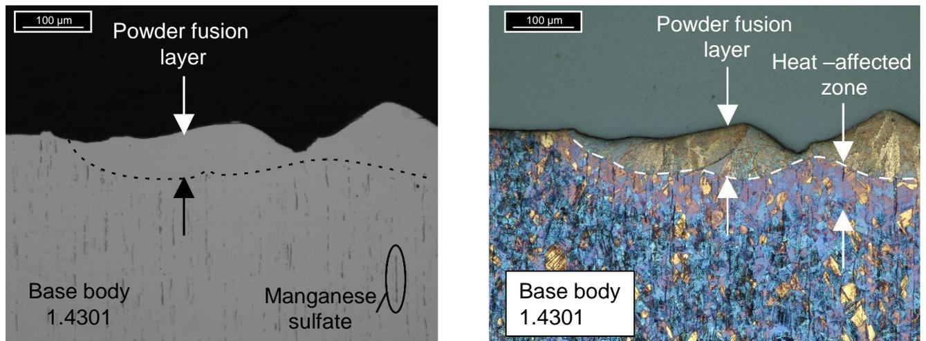
Figure 4: Polished (left) and etched (right) sample after exposure of one powder layer
