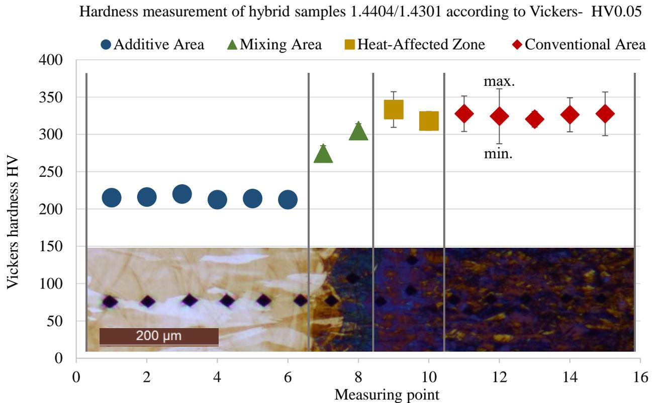
Figure 5: Vickers hardness measurement HV0.05 of the hybrid sample
