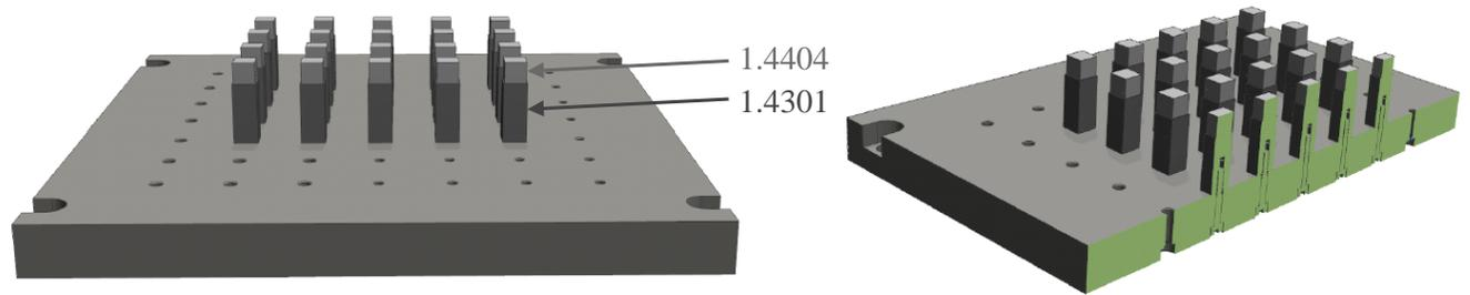
**Figure 1: Schematic illustration of the hybrid samples on the substrate plate with base bodies of 1.4301 and additive built-up volumes of 1.4404**
