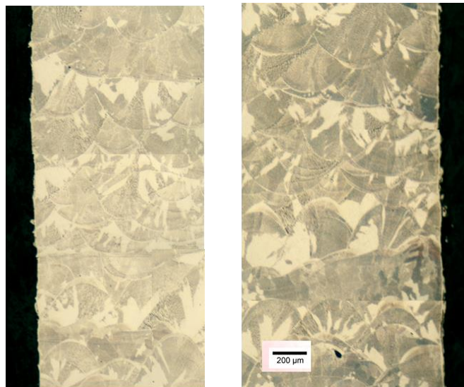
Figure 12. Both sides of bond area of sample piece observed under microscope (5X) after etching
