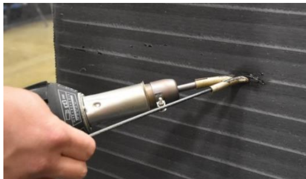
Figure 13: Re-melting polymer rods to backfill voids caused during machining
