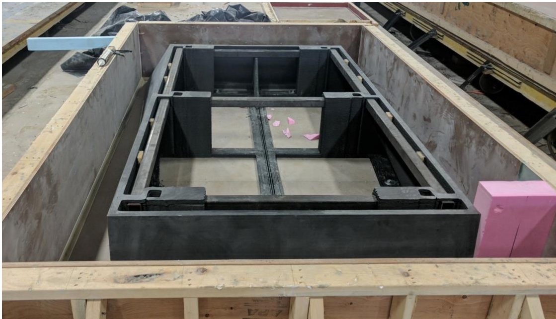
Figure 14: 3D printed mold sitting inside wooden form
