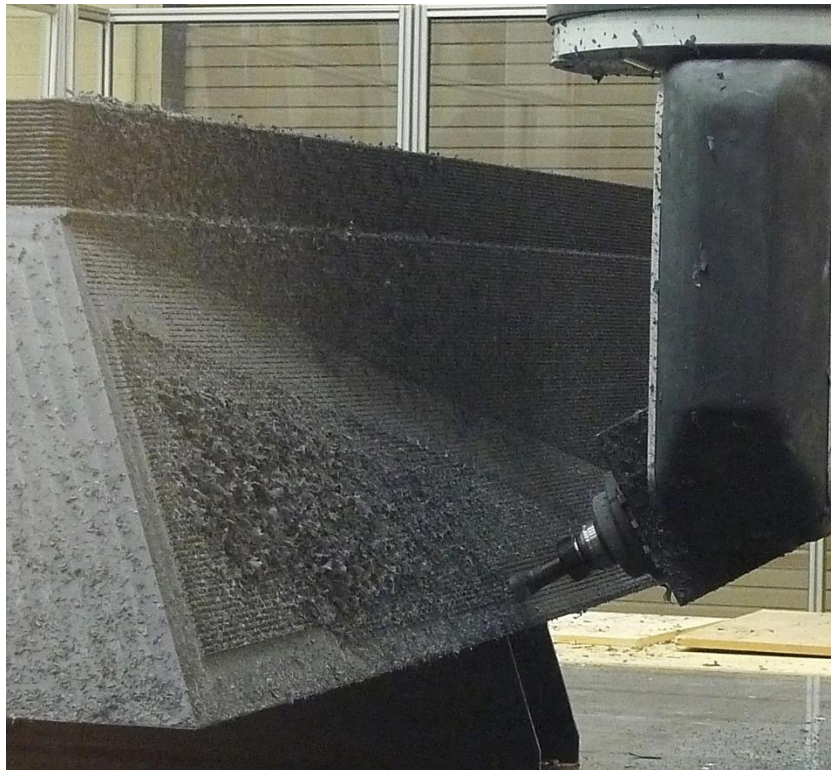
Figure 11: Machining a concrete pattern
