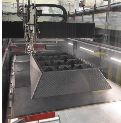
Figure 8: A mold printing inside a Cincinnati Inc. BAAM machine
