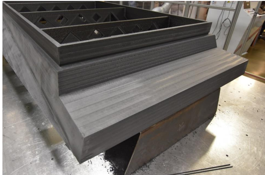
Figure 5: Concrete pattern that has an overhang exceeding 45 degrees from the vertical
