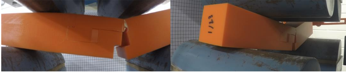
Figure 22. Four-point bending test for Kanawa-tsugi connection from two different angles
