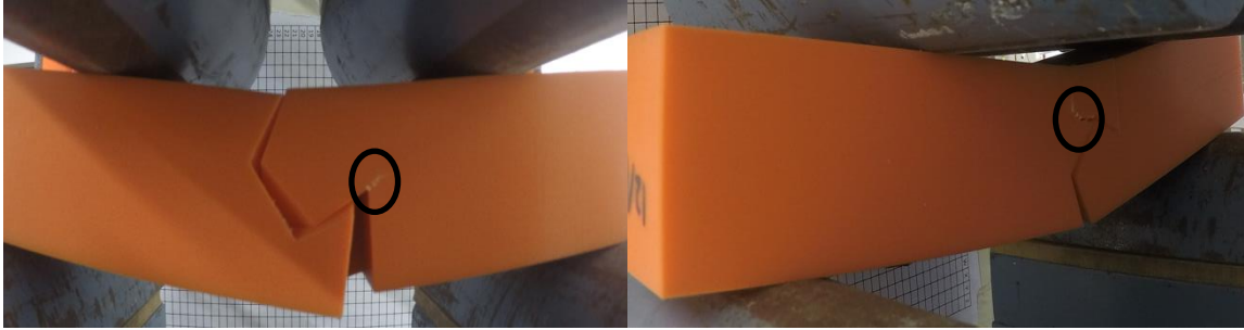
Figure 14. Four-point bending test for Kawai-tsugite connection from two different angles
