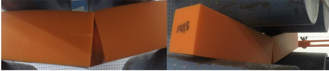
Figure 18. Four-point bending test for ConXtech from two different angles
