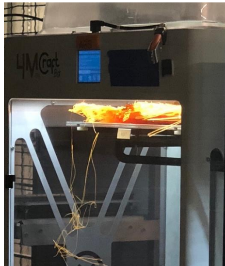
Figure 23. Failed print using ABS
