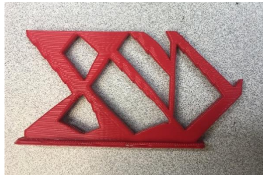
Fig 21. The corresponding printed part, with no support material, sparse infill.
