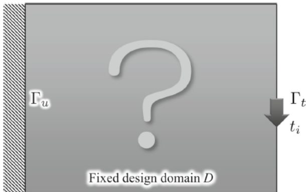
Fig 2. Design domain and boundary conditions of a TO problem.
