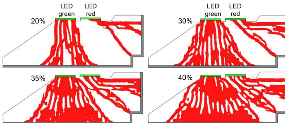
Figure 7: 2D topology optimization for the green and red LED with different mass fractions
