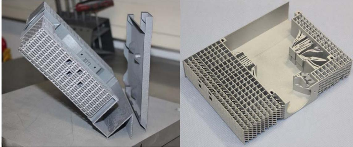
Figure 12: Projector housing manufactured by laser melting.
