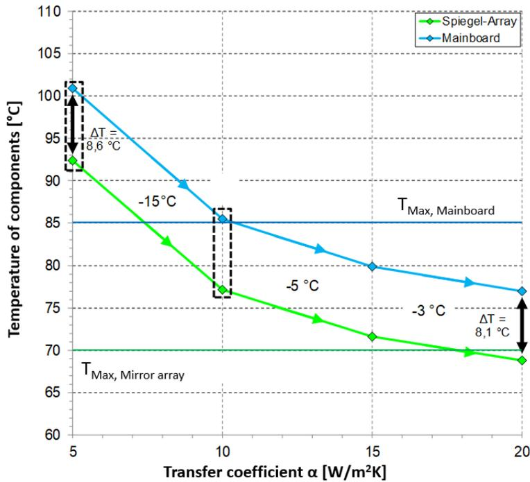
Figure 14: Influence of the heat transfer coefficient  $\alpha$  on the component temperatures
