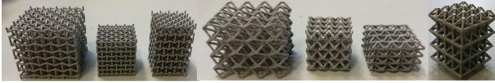
Fig.3 Some fabricated Ti6Al4V samples
