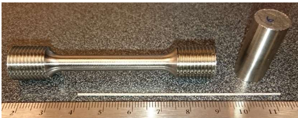
Figure 2 EBM Ti-6Al-4V specimens for testing and determination of material properties.
