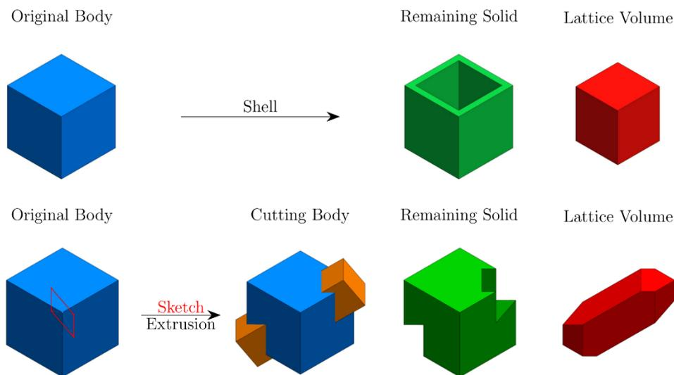
Figure 1: Definition of lattice volume – top: via shell operation; bottom: via sketch extrusion
