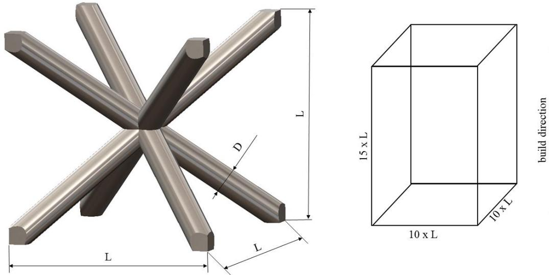
Figure 7: Compression test specimen – left: bcc unit cell; right: specimen geometry, consisting of 10x10x15 unit cells
