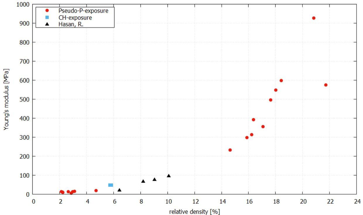
Figure 8: Young's modulus of specimens manufactured using Pseudo-P-exposure, CH-exposure, and results of corresponding tests
