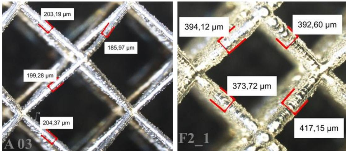
Figure 5: Differences of lattice structures manufactured with different exposure strategies but same laser parameters
