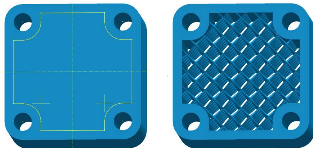
*Figure 2: Lattice design via sketch mode – left: original body with selected sketch for extrusion (yellow); right: generated lattice visualized as triangle mesh*
