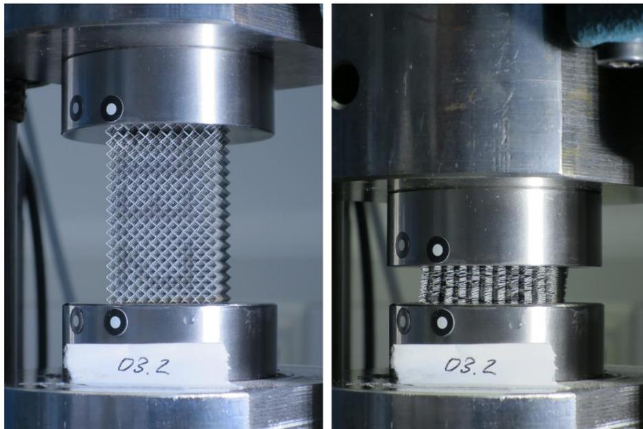
Figure 6: Compression test of specimen with  $L = 3 \text{ mm}$  and  $D = 250 \text{ }\mu\text{m}$
