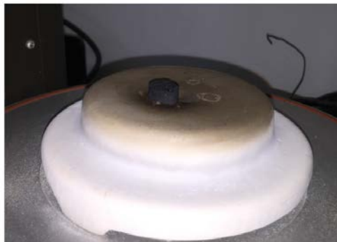
Figure 6 Resin burnout initial stages showing carbonization
