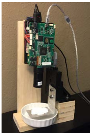
Figure 1 Final stereolithography 3D printer with all subcomponents mounted
