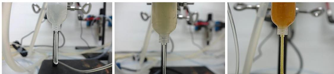
Figure 2 : Extrusion tests performed with the three compositions. From left to right: EVA/Acetone; CA/Acetone; EM/Acetone
