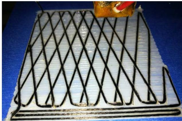
**Figure 1** 4D printing process of continuous fibers embedded Composites
