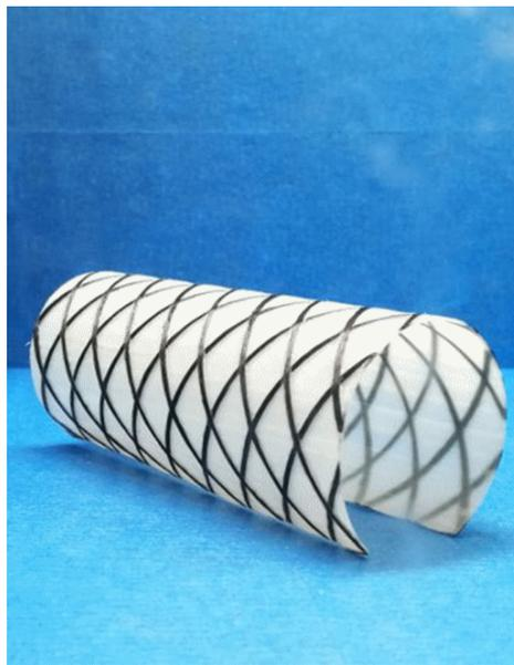
**Figure 3** The direction of the curvature is along the angular bisector between fibers
