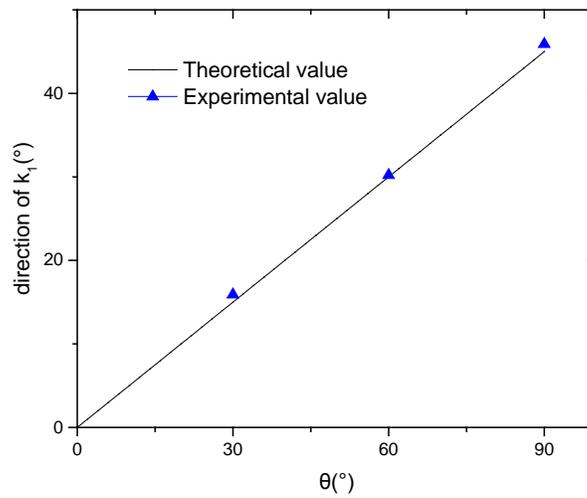
**Figure 5** The relationship between the direction of the curvature and the angle of fiber bundles
