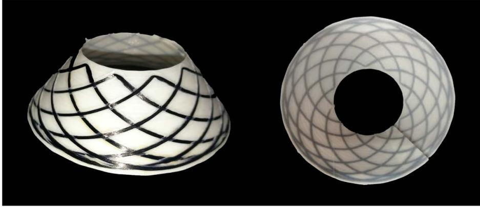
**Figure 9** The cone prepared by 4D printing
