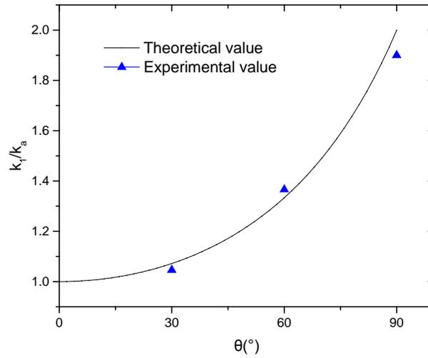
**Figure 4** The relationship between the size of the curvature and the angle of fiber bundles
