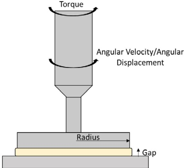
Figure 1. Model of parallel plate rheometer
