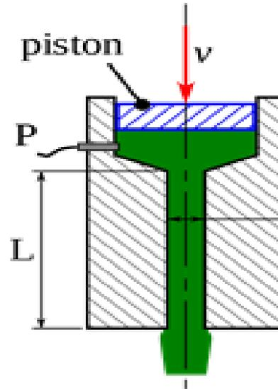
Figure 2. Model of capillary rheometer
