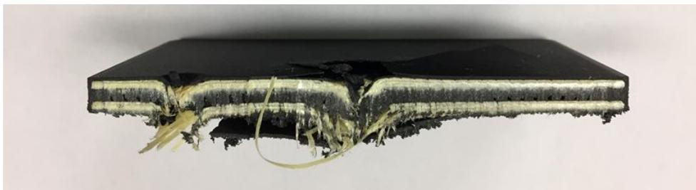
**Figure 17:** A cross section of the G3 target plate through both impact locations
