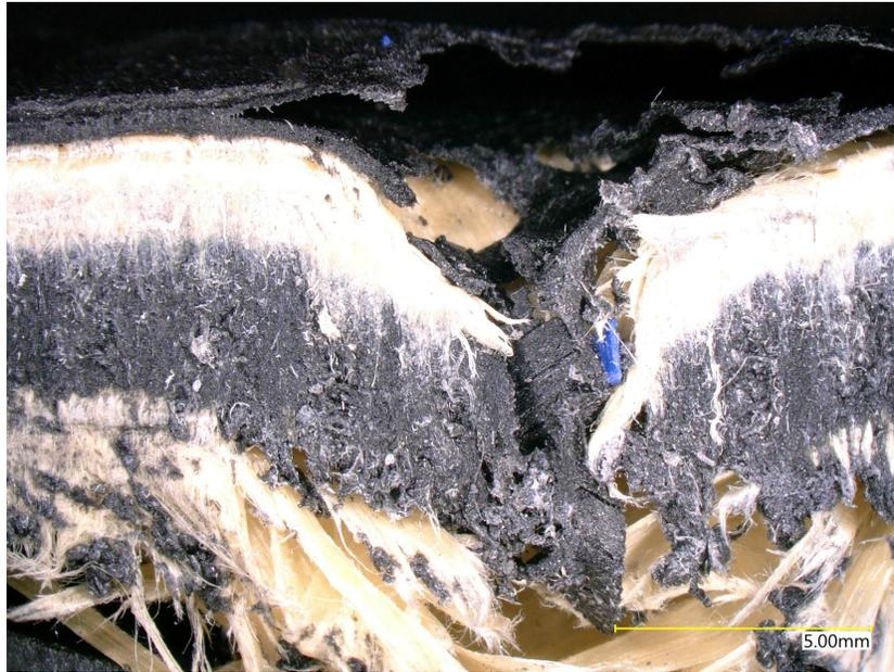
**Figure 18:** Image of the center hole (Shot #2) on the G3 sample. The blue part in the image is a fragment of the sabot.
