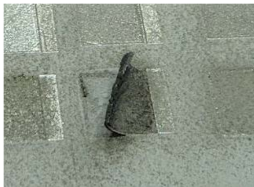
Figure 5: The consequence of large residual stress
