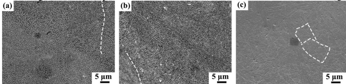
Fig. 4. SEM images of the H13 specimens of (a) without preheating, (b) 200°C preheating, and (c) wrought parts after austenitizing and tempering treatment.
