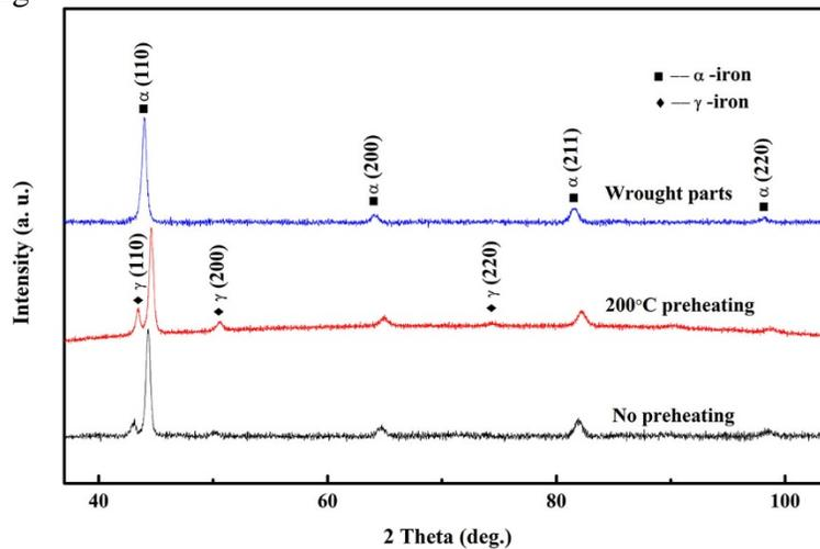
Fig. 3. The XRD spectra of H13 samples in the condition of SLM processed parts without preheating, with 200°C preheating, and wrought parts.
