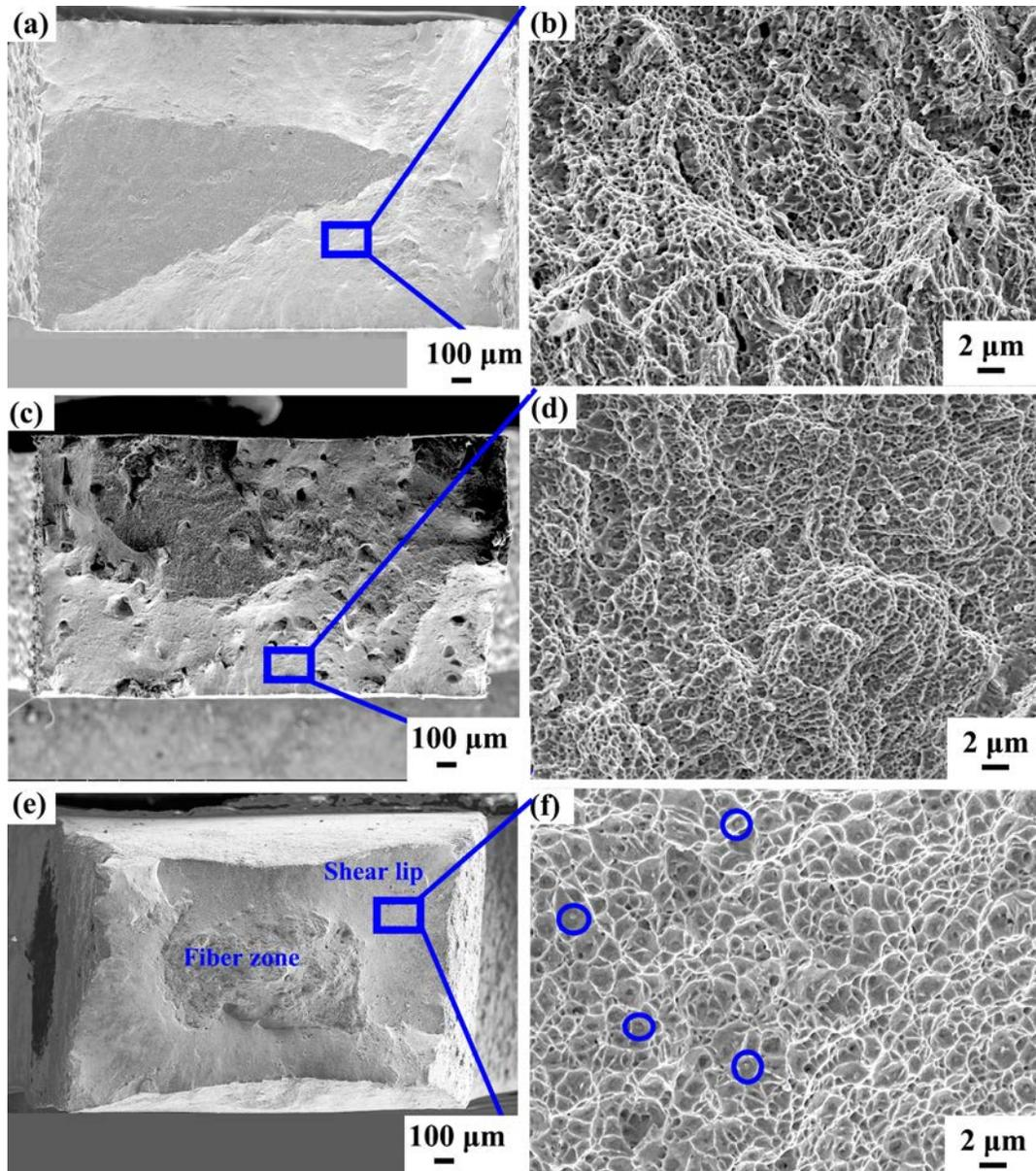
Fig. 6. SEM images of the fracture morphology of parts from tensile tests at 600°C. (a) and (b) are fracture surface of SLM processed H13 parts those without preheating. (c) and (d) are those with 200°C preheating. And (e) and (f) are wrought parts.
