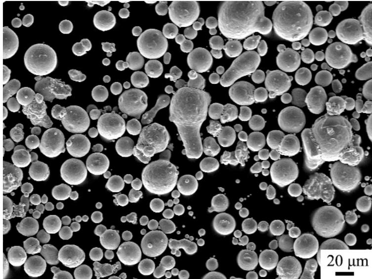
Fig. 1. SEM images of gas atomized alloyed powders.
