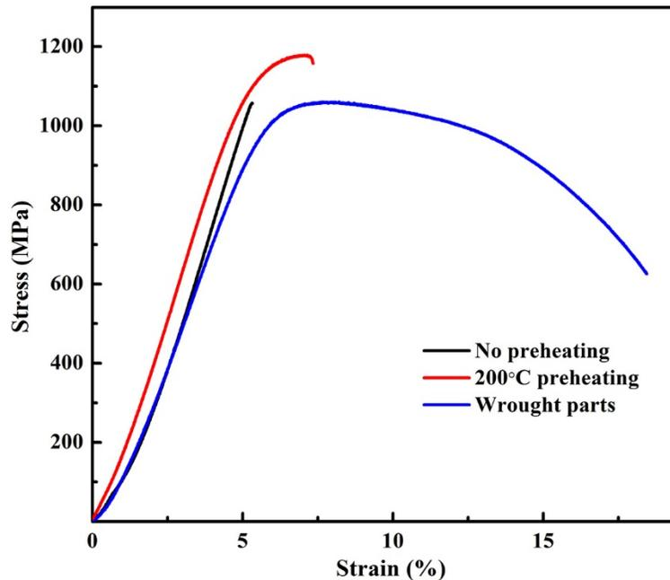
Fig. 5. Stress-strain curves of H13 samples in the condition of SLM processed parts without preheating, with 200°C preheating, and wrought parts from tensile tests at 600°C
