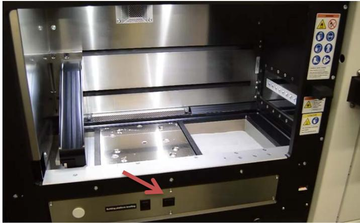
**Figure 9:** Two alignment buttons (along x and along y) are available on the front of the build chamber on EOS M290
