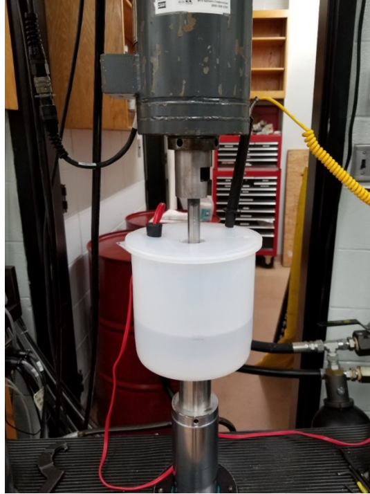
Figure 2: Test set up showing specimen submerged in solution during testing.
