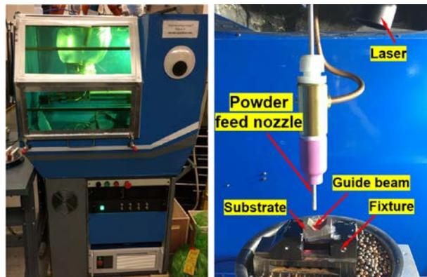
**Fig. 5** DMD system and setup
