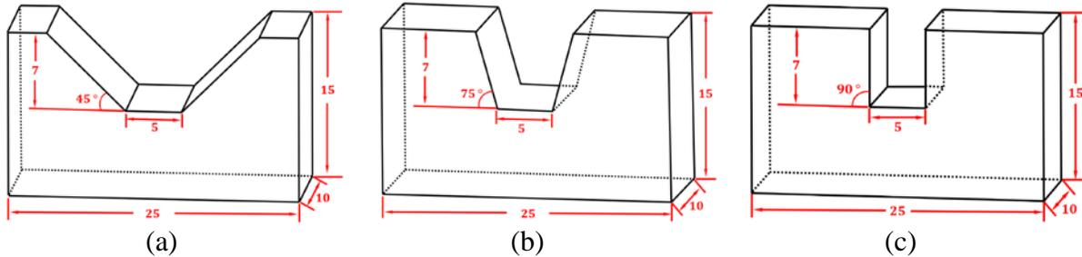
**Fig. 1** Dimensions of the prepared substrates with (a) 45°, (b) 75° and (c) 90° sidewall inclination angle
