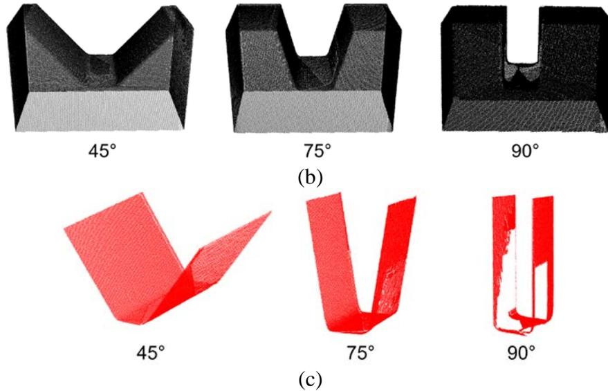
**Fig. 3** Model reconstruction for repair volume determination; (a) 3D scanning setup; (b) Reconstructed point cloud data; (c) Extracted damaged point set
