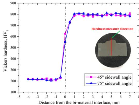
**Fig. 13** Vickers hardness tested on the cross-section of the repaired samples
