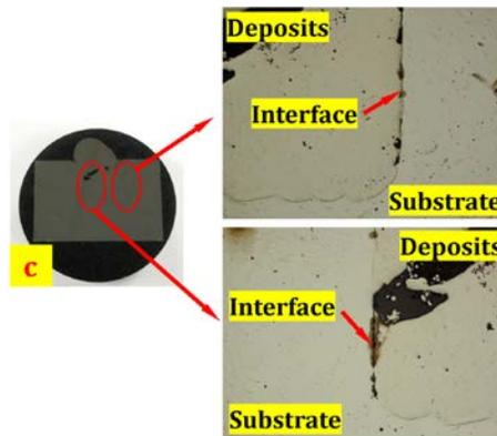
**Fig. 8** Optical micrographs of cross-sections of the repaired samples with 45° (a), 75° (b) and 90° (c) sidewall inclination angle damage
