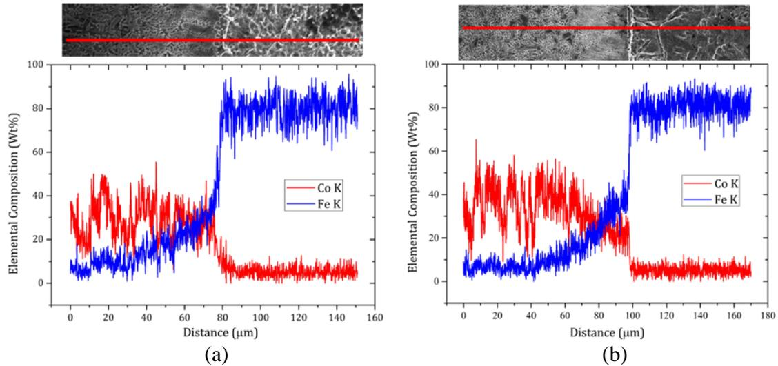
**Fig. 10** EDS line scan analysis results for samples with 45° (a) and 75° (b) damage
