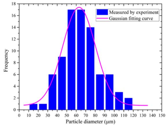
**Fig. 2** SEM micrograph (a) and particle size distribution (b) of Wallex 50 powder
