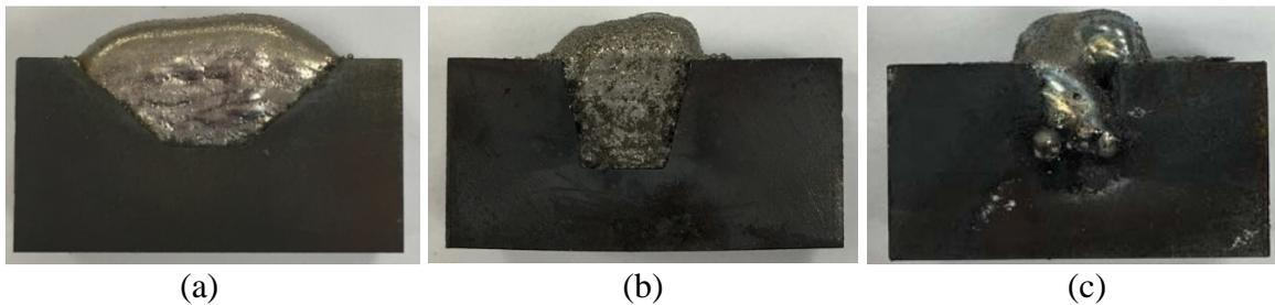
**Fig. 7** Overview of the repair samples with  $45^\circ$  (a),  $75^\circ$  (b) and  $90^\circ$  (c) sidewall inclination angle
