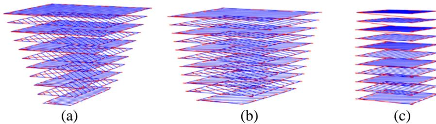
**Fig. 4** Repair tool path for substrates including defects with (a) 45°, (b) 75° and (c) 90° sidewall inclination angle
