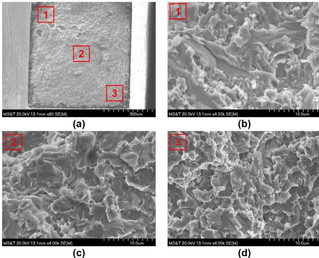
**Fig. 12** Tensile fracture morphologies; (a) Overview of the fracture surface; (b) Magnified view of area 1 in (a); (c) Magnified view of area 2 in (a); (d) Magnified view of area 3 in (a)
