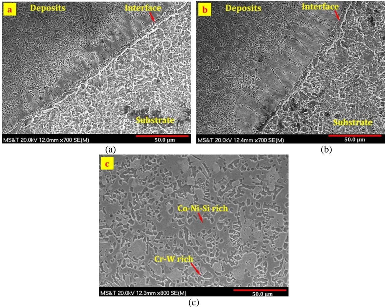
**Fig. 9** SEM micrographs of the boundary area of repaired samples with 45° (a) and 75° (b) sidewall damage; (c) Micrographs of top layers of the repaired sample with 45° sidewall damage
