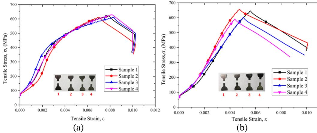
**Fig. 11** Tensile stress-strain curves for repaired samples with 45° U-shaped defects (a) and 75° U-shaped defects (b)
