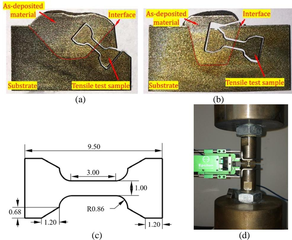
**Fig. 6** Tensile test specimen preparation and setup; Tensile specimen over the sectioned repaired substrates with 45° (a) and 75° (b) sidewall inclination angle damage; (c) Dimensions of the tensile test specimen (Dimensions in mm, 1mm in thickness); (d) Tensile test setup
