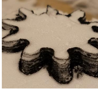
Figure 1. Partially sintered sample with weak bonding between layers
