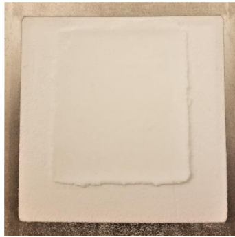
Figure 2. Warpage caused by cumulative heating
