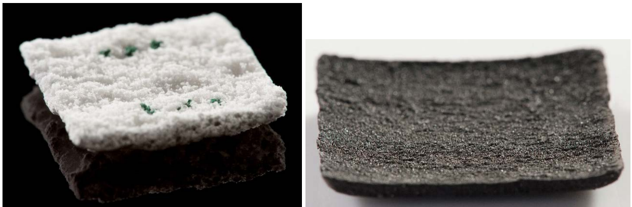
Figure 8 – Left: laser sintered PCTFE. Right: laser sintered PCTFE 1 wt% CB part, 20 x 20mm.
