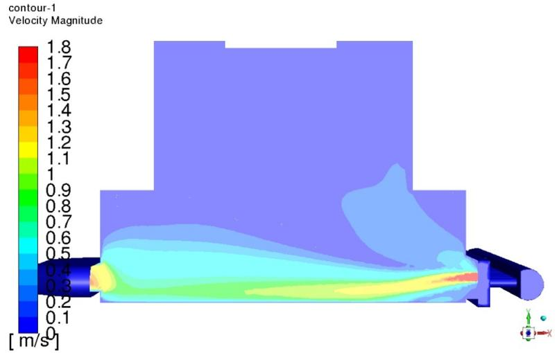
Figure 11, Side view of velocity contour for the optimized design with downward secondary flow
