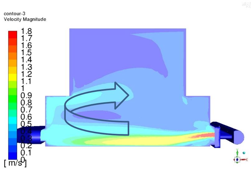
Figure 10, Side view of velocity contour and recirculation for the optimized design
