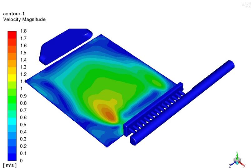
Figure 8, Velocity contour on the plane 3mm above the bottom for the extended nozzle array design
