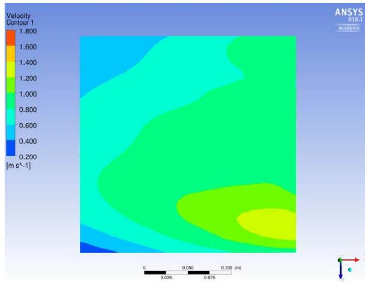
Figure 6, Velocity contour on the plane 3mm above the build plate for the design with reduced nozzle height and elongated length
