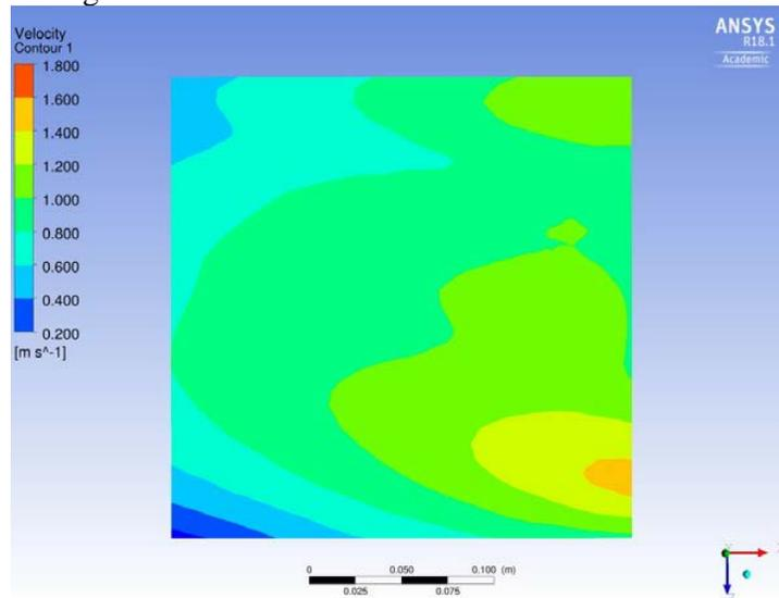
Figure 6, Velocity contour on the plane 3mm above the build plate for the design with reduced nozzle height
