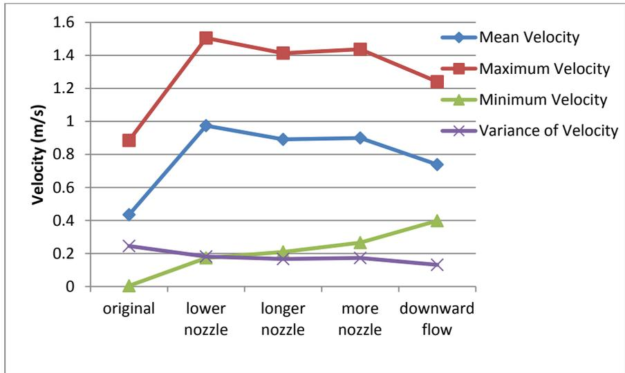
Figure 12, Evaluation of uniformity of flow velocity for design optimization step by step
