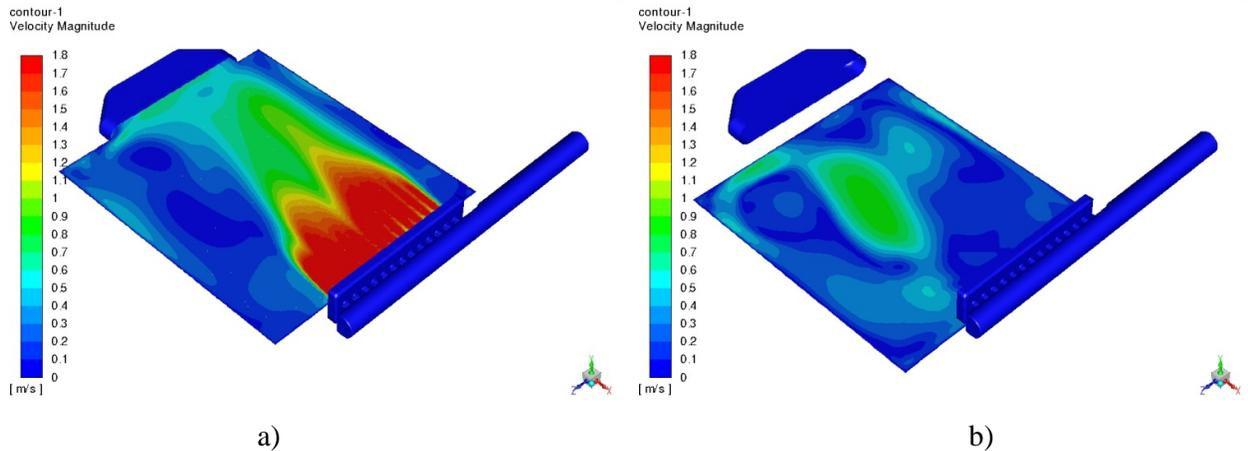
Figure 3, Velocity contour on the plane through the inlet nozzle's center a) and the plane 3mm above the bottom of chamber b) for the original design
