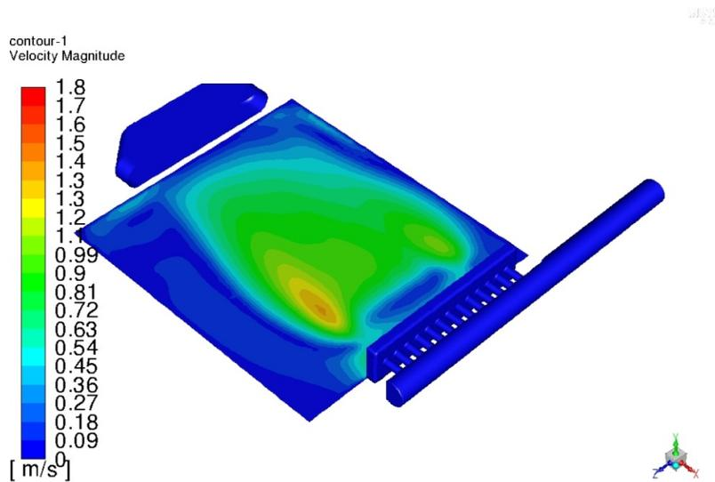
Figure 7, Velocity contour on the plane 3mm above the bottom and sweeping down jet at the ends of nozzle array
