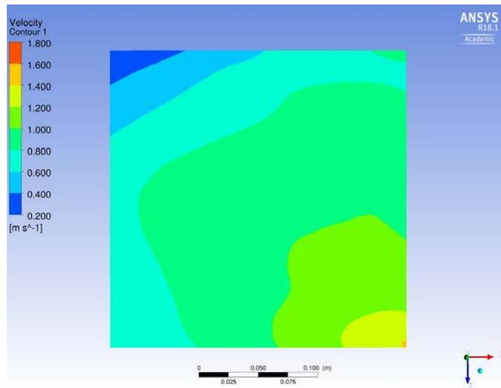
Figure 9, Velocity contour on the plane 3mm above the build plate for the design with extended nozzle array
