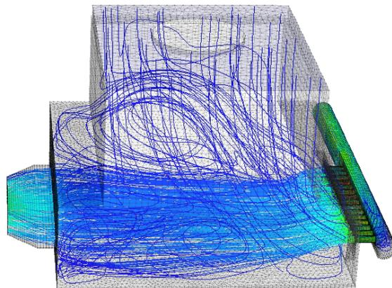
Figure 12, Path lines of gas flow for the optimized design with downward secondary flow
