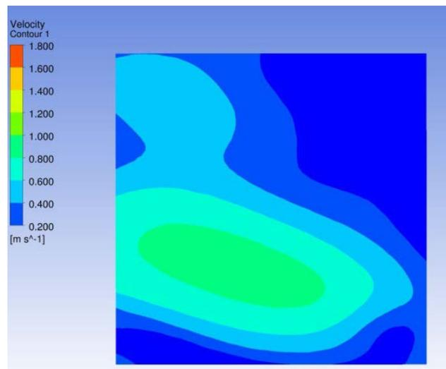
Figure 4, Velocity contour on the plane 3mm above the build plate for the original design
