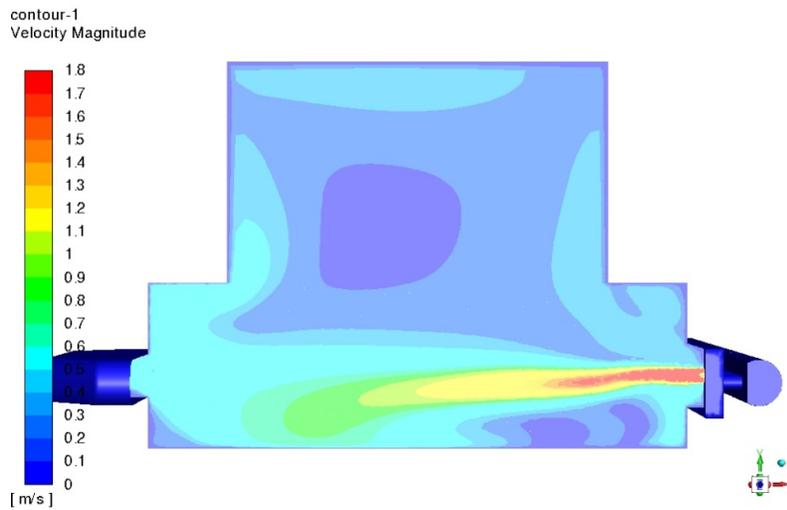
Figure 5, Side view of velocity contour of jets for the original design
